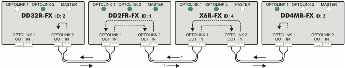
**Fig. 1: A non-redundant network with one DD4MR-FX unit**
