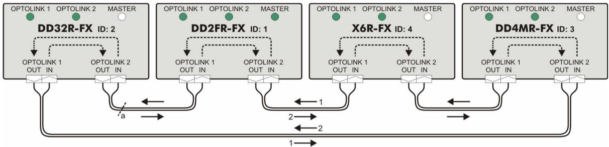
**Fig. 2: A redundant network with one DD4MR-FX unit**
